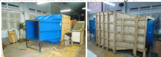
Figure 6. The finished wind tunnel: viewed from the nozzle (left) and from the inlet section (right).
