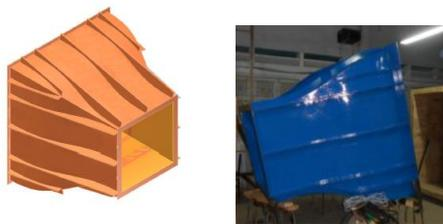
Figure 5. CAD model (left) and fabricated contraction (right).
